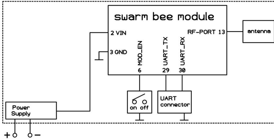
Figure 3-1 autonomous tag without host controller
