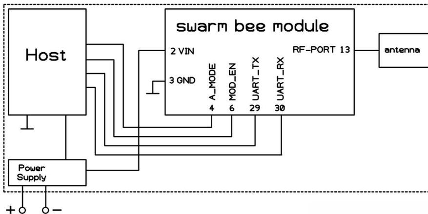
Figure 3-2 tag with host controller
