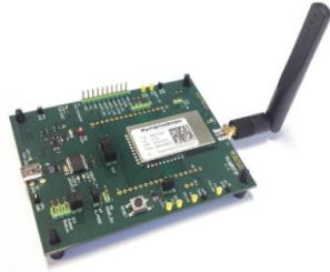
Figure 2: swarm bee DK+ Boards in three variants: DK+ LE V2 or V3 (Chirp) and DK+ ER (UWB)
