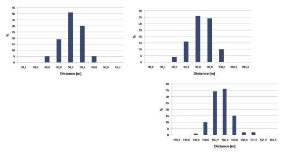
**Figure 5 Ranging Accuracy -** Ranging Accuracy is characterized by offset and spread. The actual distances are 50, 100, and 150m respectively
